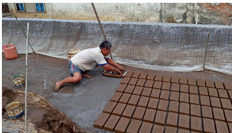
Figure 3.2 Brick making process
